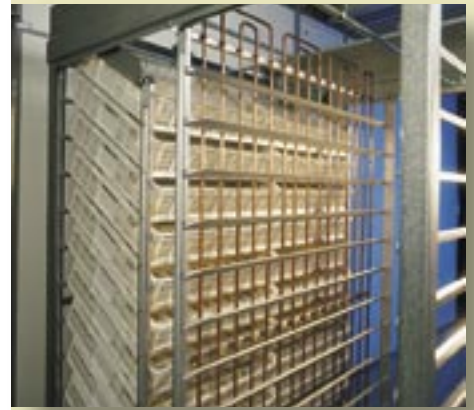
Each single-stage setter trolley has its own heating/cooling element
