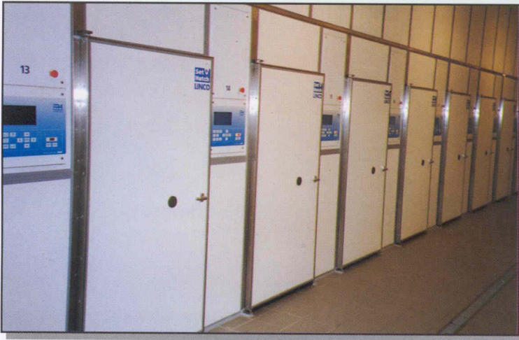
The Linco Set and Hatch hatchers. Note the operator friendly control panels and, below right, how the internal design facilitates easy cleaning.
