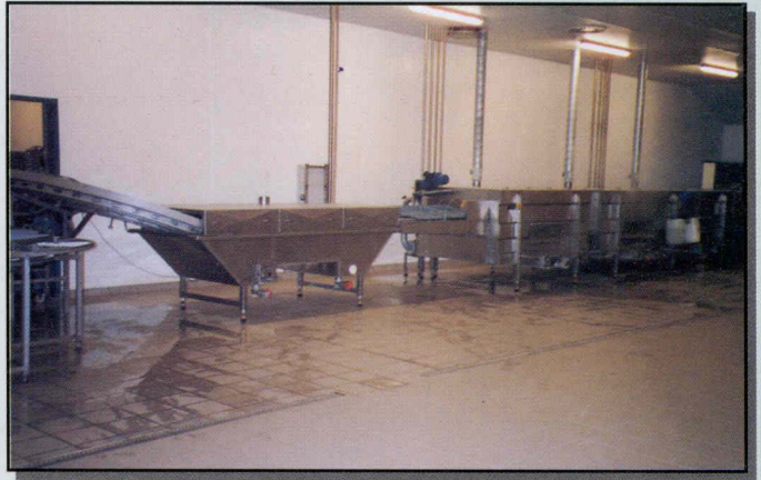
Cleaning of trays and boxes is an important task. For the boxes this starts, above left, with a pre-soak. The firm that manufactures this equipment, Linco, also manufacture water rides for theme parks! Another important aspect of hygiene is the removal of any dust or fluff from eggs or chicks (see below left).
